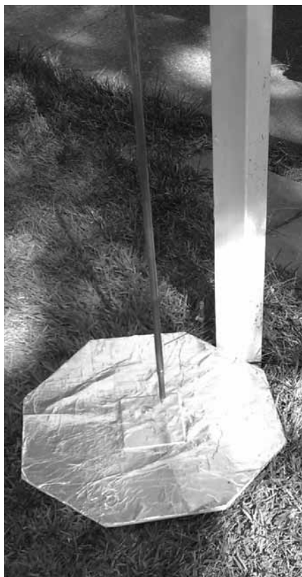
Photo 7 — The All-Band Antenna measurement setup is shown in these photographs. On the left it is being operated only as a simple vertical with good grounding. For the photograph on the right the SWTL launchers and VHF+ antenna are present. In addition to the hexagonal aluminum foil disk, which provides a good VHF ground, an 8 foot ground rod near the wooden post is also connected to the disk. This arrangement was left in place for all measurements even though the disk is not necessary when the launcher is in place.
