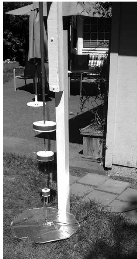
Photo 7 — The All-Band Antenna measurement setup is shown in these photographs. On the left it is being operated only as a simple vertical with good grounding. For the photograph on the right the SWTL launchers and VHF+ antenna are present. In addition to the hexagonal aluminum foil disk, which provides a good VHF ground, an 8 foot ground rod near the wooden post is also connected to the disk. This arrangement was left in place for all measurements even though the disk is not necessary when the launcher is in place.
